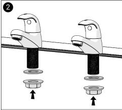
Whilst holding the tap in place, screw the nut and washer onto the tap tail and tighten. Do not overtighten as this may damage the mounting surface.
