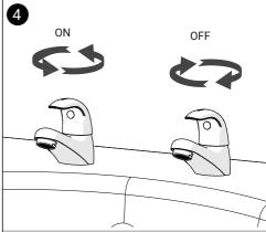
**Commissioning:** Turn the cold tap on. Allow a few minutes of running to flush the system and then repeat for the hot water. Then turn off.
